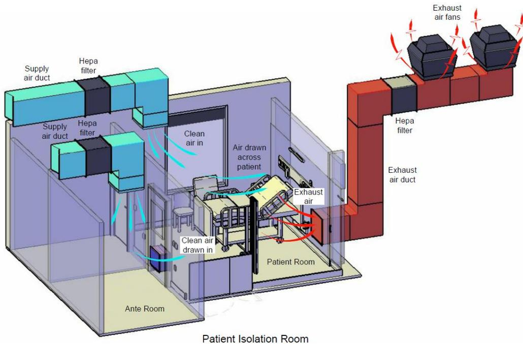
The concept is relatively simple, refer schematic representation above, in that an amount of conditioned air (heated or cooled and/or humidified and filtered) is supplied into a well-sealed room, with a higher quantity of air being extracted out of the room at all times.
